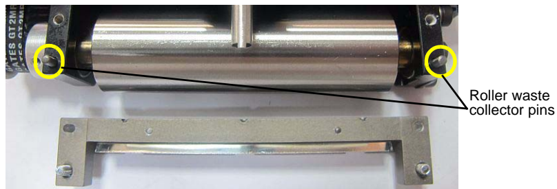
Figure 6-36: Roller waste collector pins
