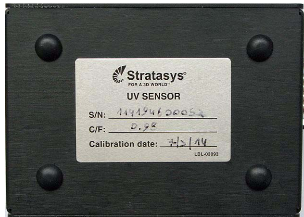
Figure 6-85: Label on the bottom of the UV sensor
