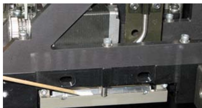
Figure 6-35: Cleaning the roller waste collector
