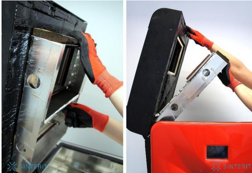
Photo 9. Correct holding unit heaters while loosening
