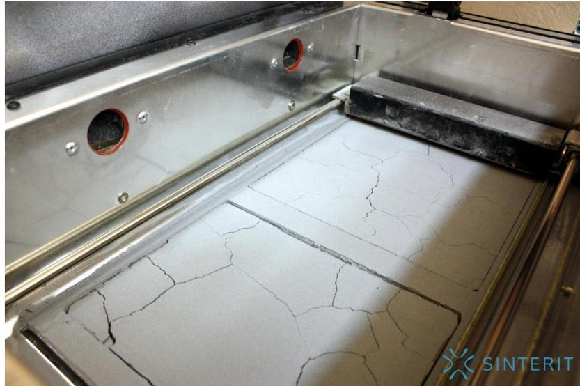
Photo 21. The correct state of powder after printing (visible cracks on the surface of both BED)
