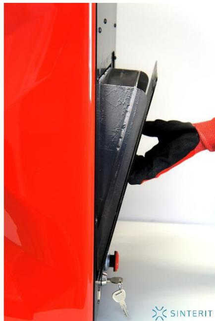
Photo 21. Correct removal and insertion the OVERFLOW BIN
