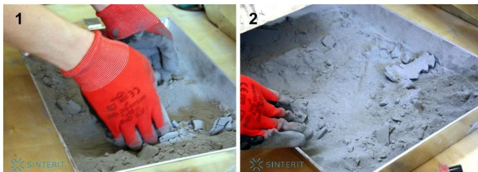
Photo 26. The method of crushing the remnants of print and pre-sieving
