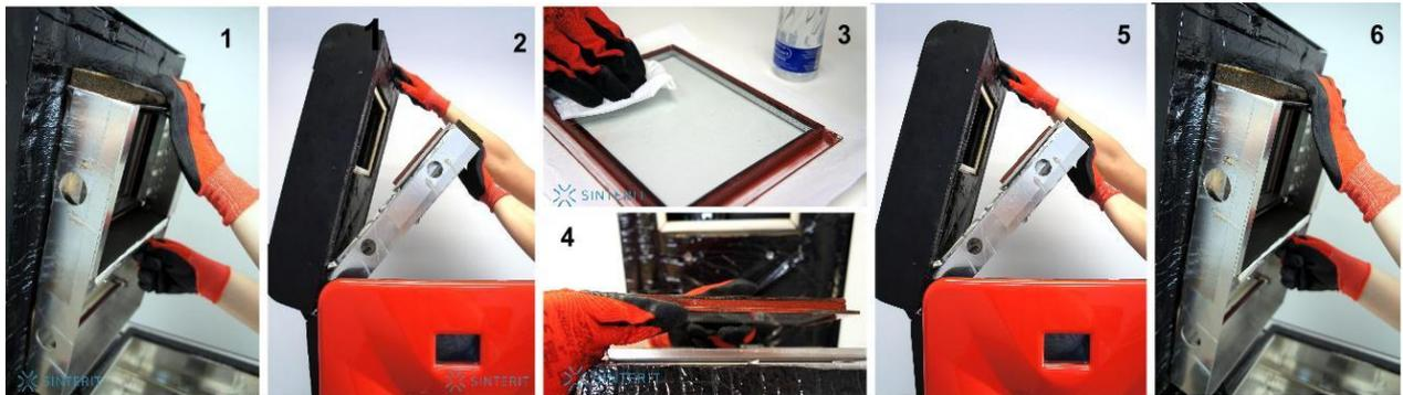
Photo 28. Replacement of the glass protecting laser
