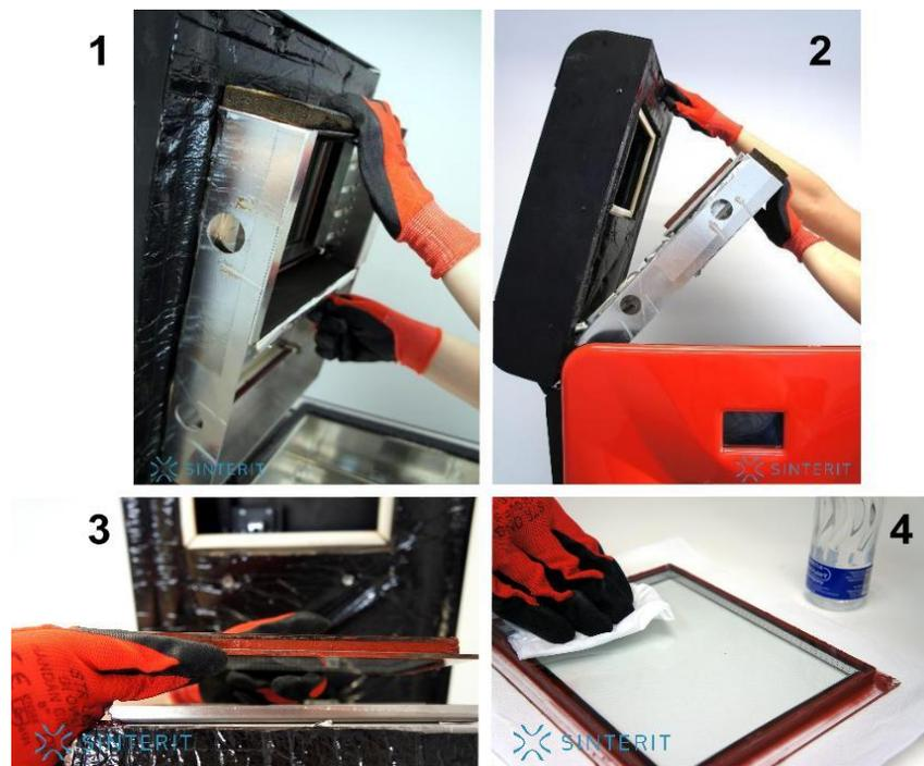
Photo. 24. Cleaning the protective glass laser
