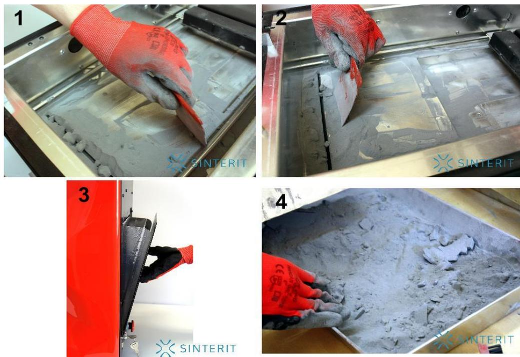
Photo 23. Removing the remaining powder from inside
