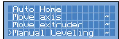
Level the bed on positions: 1, 2, 3, 0 by means of the external wheels placed under the bed.
