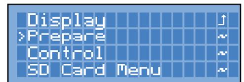
According to the filament type, select the correct pre-heating function (the ABS option is correct also for different filaments such as Nylon or Polystyrene).
