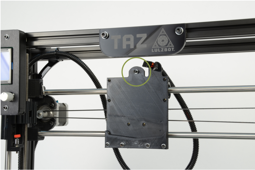
Figure 1.11: Remove the tool head screw
