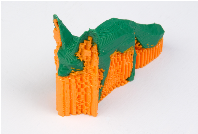
Figure 5.17: An example of an object printed with support material.
