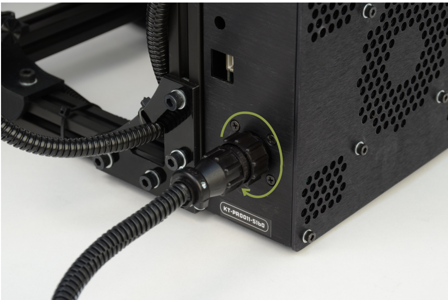
Figure 1.17: The power supply plug correctly plugged in
