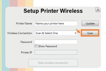
8 Use the pull-down menu to view a list of Wi-Fi connections available in the area, and select the Wi-Fi connection that you wish to connect to.
