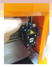
3 Ensure that the guide tube is properly inserted into the feed port of the extruder module to complete the installation.
