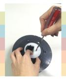
Use a phillips screwdriver to loosen the securing screws of the filament spool ring.
