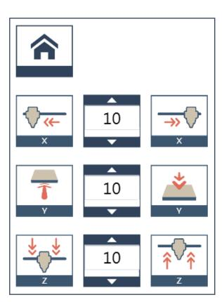
Manually adjust the movement of X/Y/Z Axis for printer maintenance.
