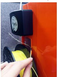
Note: The end tip of the ejected filament may exhibit some residual effects. This is considered a normal phenomenon.
