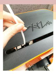
2 Feed the guide tube through the slot at the top of the printer to the extruder module.
