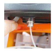
5 Press the release arm and push the filament all the way to the bottom so that the front end of the filament is completely inserted into the extruder module.
