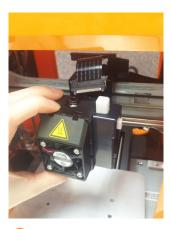
1 Make sure that the printer is powered off. Place the extruder module that the fitting pin is secured the proper location.
