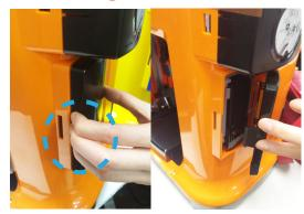
Remove the side cover by pressing down firmly at the center on the left side of the cover and pushing aside the cover. (pay attention to where you apply your force to ensure proper dismantling) Keep the side cover securely for future use.
