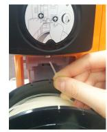
Take the tip of the filament and insert it into the feeding hole.
