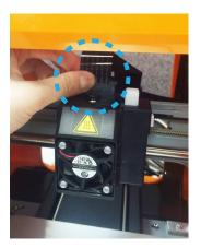
2 Insert the black ribbon connector to complete the installation.
