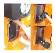
Lower the filament spool holder on the left side of the printer until horizontal.
