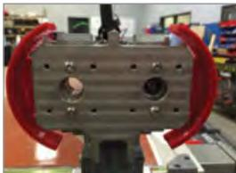
4. Y axis bumper protects the user from contact with the idle end of the actuator during printing
