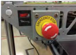
5. (2) Emergency Stop buttons located on the front and back of the machine
