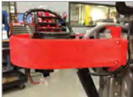
3. Y axis bumper protects the user from contact with the motor end of the actuator during printing
