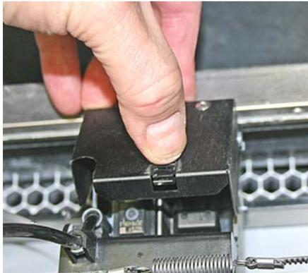
5. Lift print head out of its slot and properly recycle or dispose of the empty cartridge. On a ProJet 260C, ALSO remove the other printhead even if it does not need replacing.
