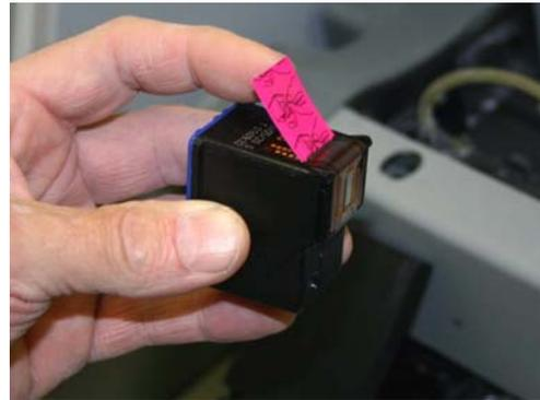
11. Insert the new printhead. Press down firmly on the top of the printhead, at the same side as the pogo pins, to securely fit the printhead into its slot.
