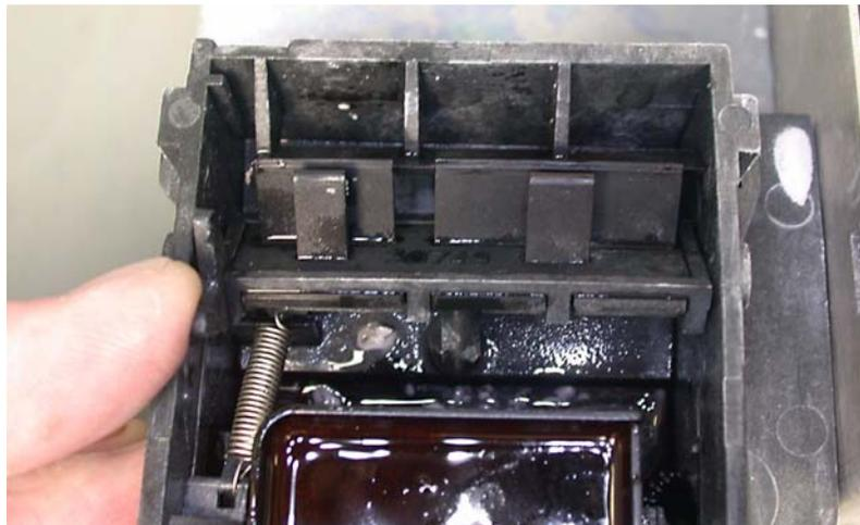
4. Position the squirt bottle close to the station and squirt water into the service station.
