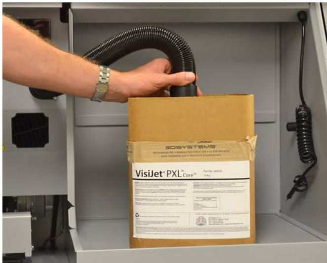
4. Select **VACUUM** on the LCD menu. The vacuum starts. Direct the nozzle inside the container so it pulls up a continuous stream of Core material.
