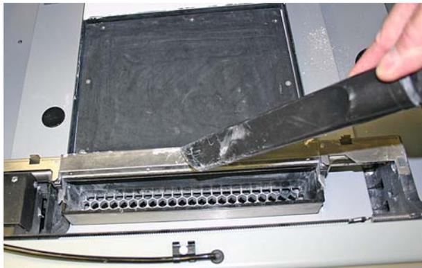
5. The vacuum will stop automatically if the Feeder becomes full, or you can push the Control Knob once to shut off the vacuum. If the Feeder does become full, the LCD displays:
