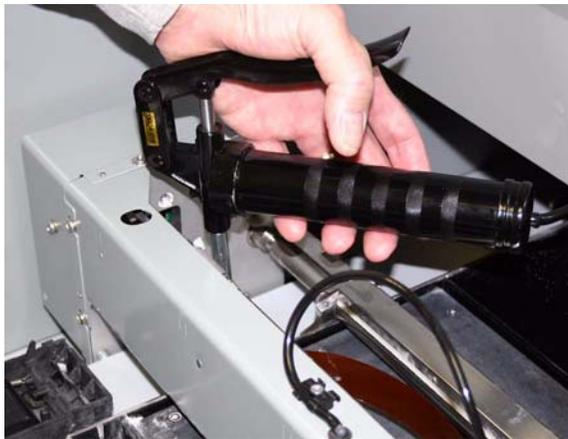
7. Squeeze the trigger 2 - 3 times or until you feel the tension change and then **STOP**. *Do not over-grease.*
