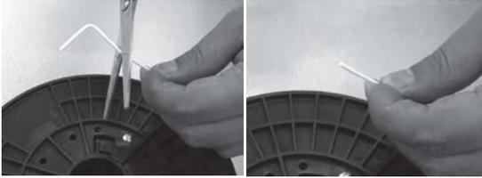
7.2.1.2 Push down the Printer Head arm. Insert the filament into the hole located on the top of the the Printer Head. Push the filament until the tip of the filament is inserted into the nozzle receiving port. Then release the Printer Head arm.
